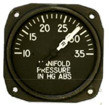
The more air and fuel that is drawn into the cylinders, the more power the engine can develop, and the air pressure in the induction system, just before the air / fuel mixture enters into the cylinders, gives a good idea of how much power is being developed.
