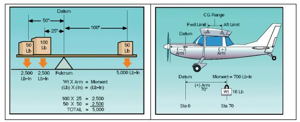
We need to calculate the moment of each element (taking the empty aircraft with no fuel as one element) from the datum and add them all together.
