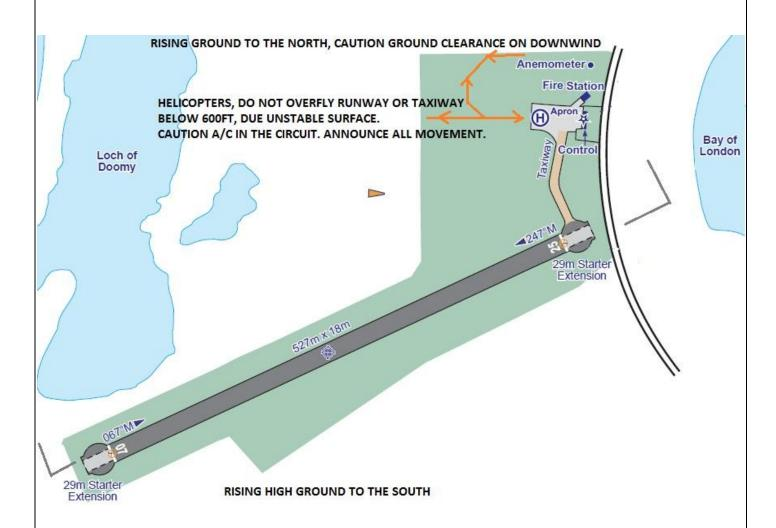
THIS A/F IS NOT RECOMMENDED FOR USE BY LOW WING A/C OR A/C WITH SMALL PROPELLER GROUND CLEARANCE, DUE TO THE UNSTABLE HARDCORE SURFACE OF MAIN RUNWAY AND TAXIWAY. POWER CHECKS SHOULD BE CARRIED OUT, WITH, CARE, ON THE ASPHALT APRON.
