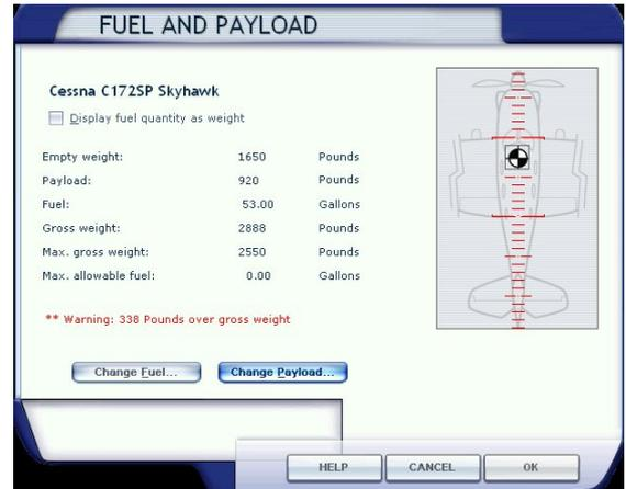
The two illustrations above show the effect in FSX of our four 15 stone passengers and their luggage with full fuel tanks. Note that although significantly overweight, the centre of gravity remains well within limits.
