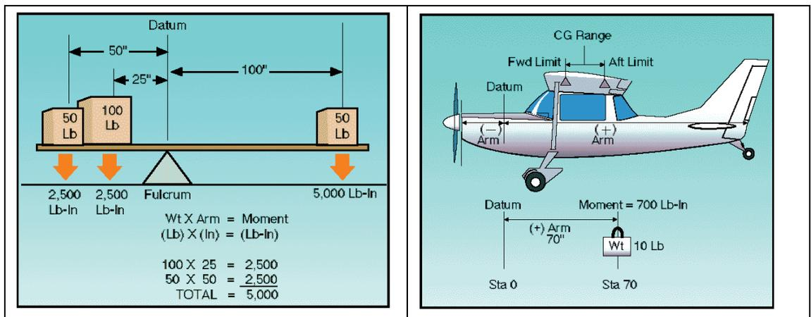
We need to calculate the moment of each element (taking the empty aircraft with no fuel as one element) from the datum and add them all together.
