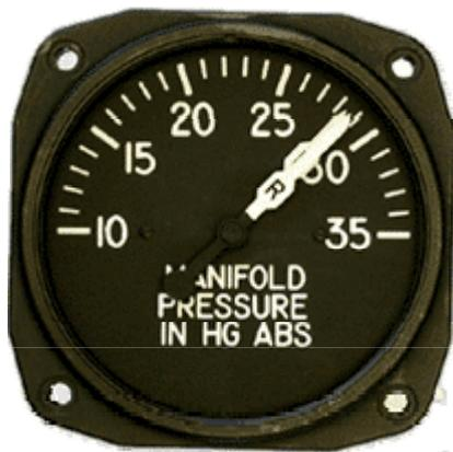
The more air and fuel that is drawn into the cylinders, the more power the engine can develop, and the air pressure in the induction system, just before the air / fuel mixture enters into the cylinders, gives a good idea of how much power is being developed.
